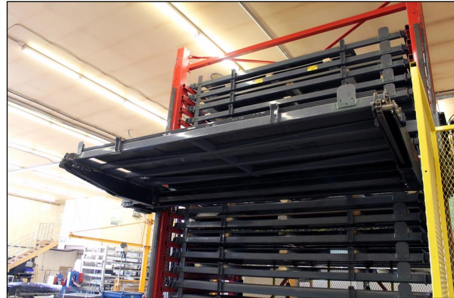
Vidir's VLS will store and retrieve material, utilizing available overhead space and deliver product to ground level for further processing and integration with production machines.
